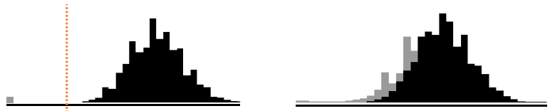
Figure 6. Left: a threshold (dotted vertical line) separates attack values (grey) from normal values (black). Right: attack values mimic the distribution of normal values. Adapted from [39].
